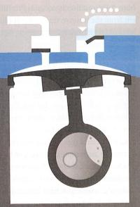
FIGURE 1: In a diaphragm pump, a diaphragm moves up and down in a chamber, and inlet and outlet valves are used to transfer liquids.
